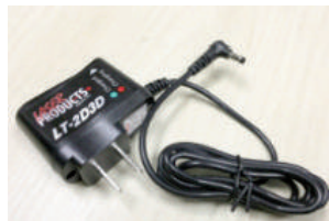
LT-2D3D Laser Templator Power Supply
